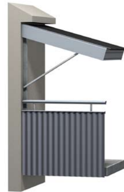
Standard roof with braces anchored in the steel posts.
