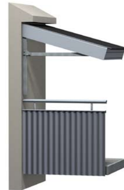
Cantilever roof fixed directly into the wall.
