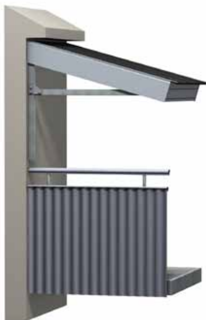
Cantilever roof fixed directly into the wall.
