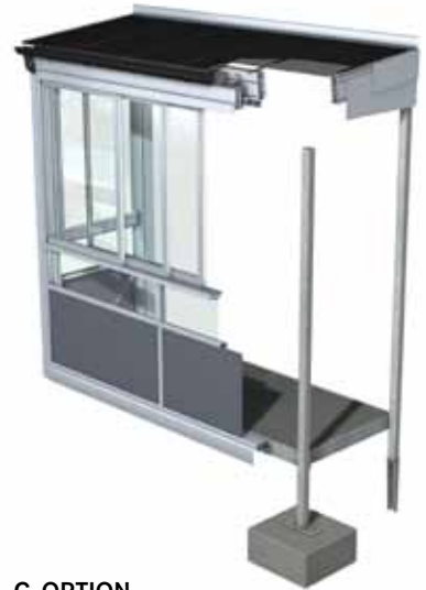
C. OPTION Post at front edge on new foundation. Fixing to building carcass along back edge.
